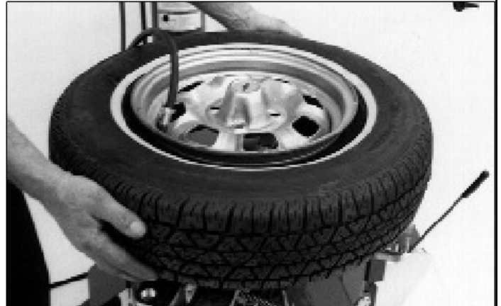
Figure 19 - Lift Tire Upwards for Bead Sealing
