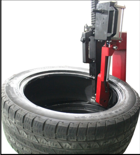
11.1 first install bottom bead tip on the rim.
